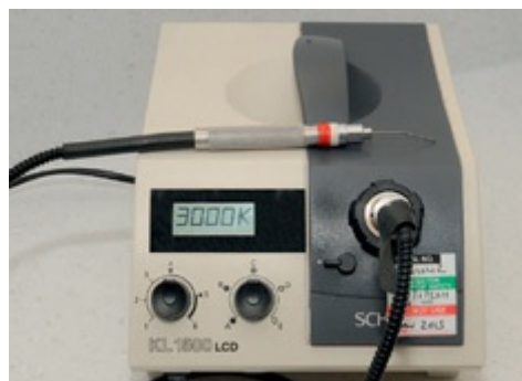
Figure 6.10 A portable FOTI light source with a 0.5mm diameter tip. As dental headpieces contain fibre-optics these are often incorporated into the dental unit.
